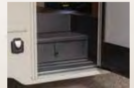
Integrated entry step with 80" entry door and auxiliary battery box.
